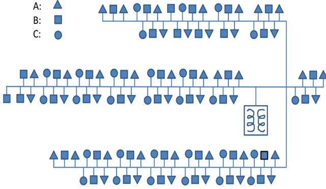
Figure 1. A diagram of an Victorian suburban distribution network of 114 houses fed by a 300kVA distribution transformer. Triangles denote houses on phase A; rectangles denote houses on phase B and circles on phase C.
