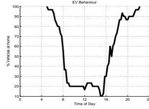
Figure 2. An average workday EV travelling profile generated from a sample of size 100 from of EV trial project database.
