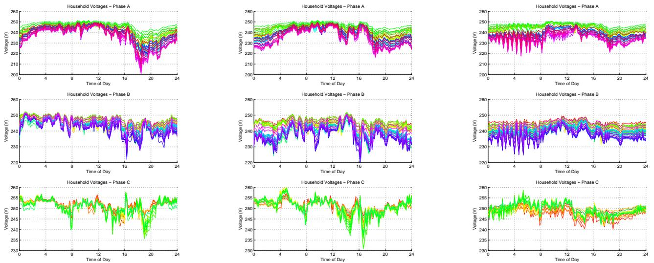
Figure 5. The household local voltage levels of the uncontrolled charging (first column), centralized charging (second column) and distributed greedy fair charging (third column). The first three rows show the voltage of individual houses on individual phases; each color denotes a house.
